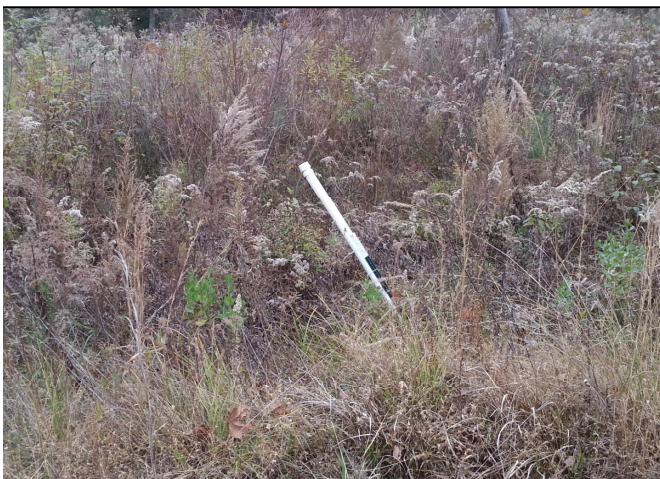
Photo 3: Crest Gauge (Main East) Leaning Over Following Bankfull Event - Fall 2013
