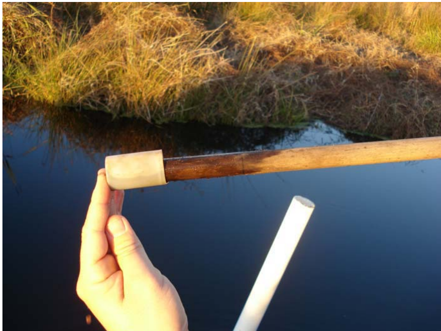
Photo 4. Crest gauge showing water above bankfull (11/16/07)
