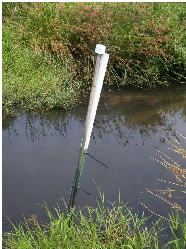
Photo 4. Crest gauge showing water above bankfull (7/03/08)
