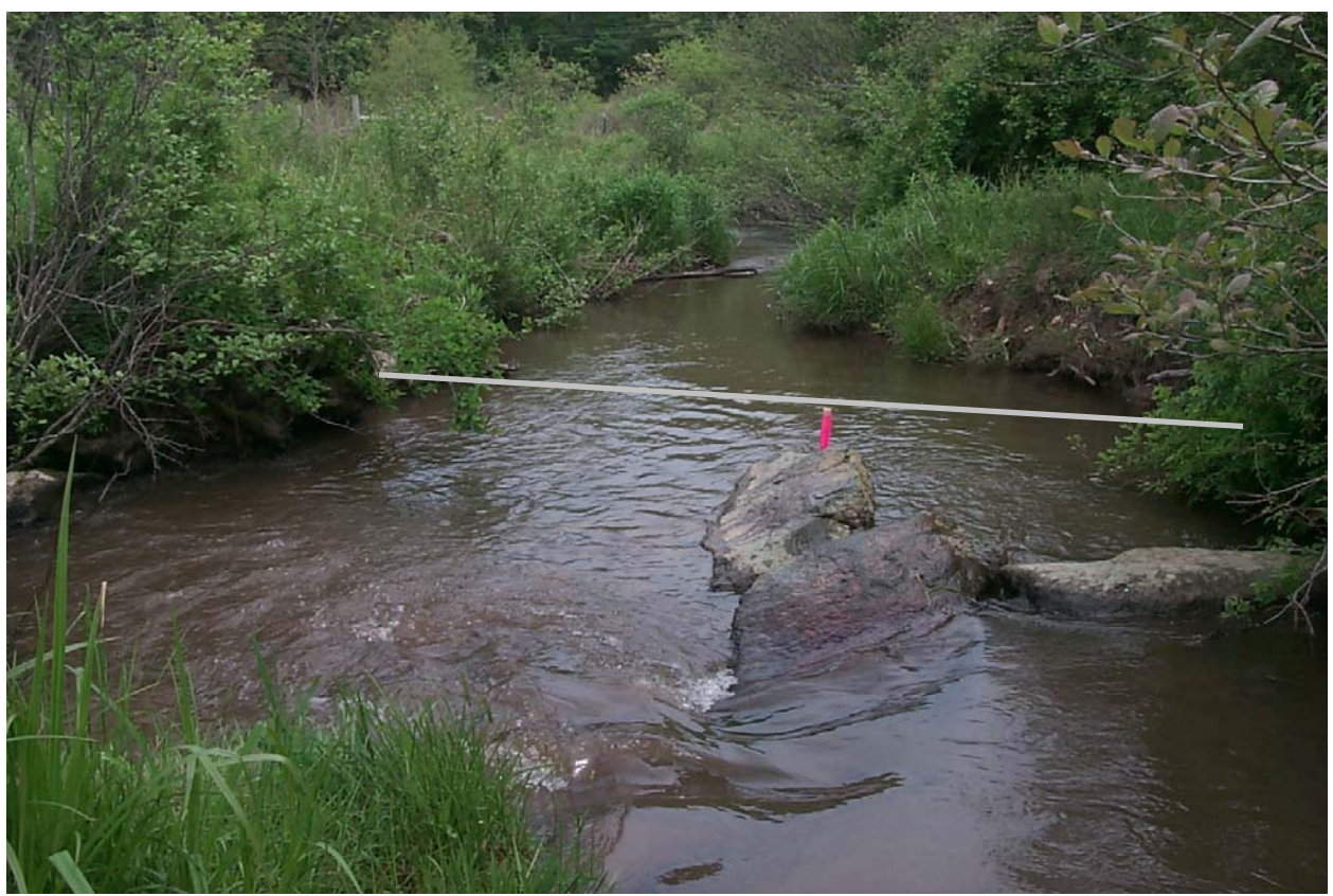
FIGURE 3.7.—Cross-section station 12+74, pool.
