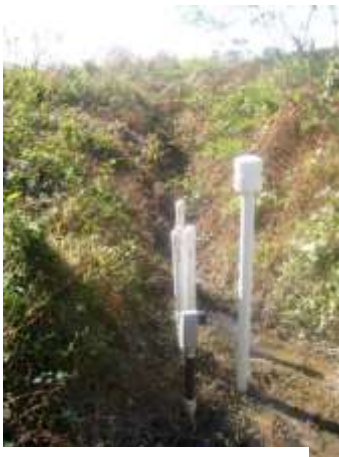
Monitoring wells used to collect hydrologic data to determine success of restoration projects.
