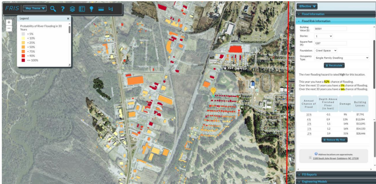
Figure 3-5: FRIS displays regulatory flood hazards and probability/damage estimates.
