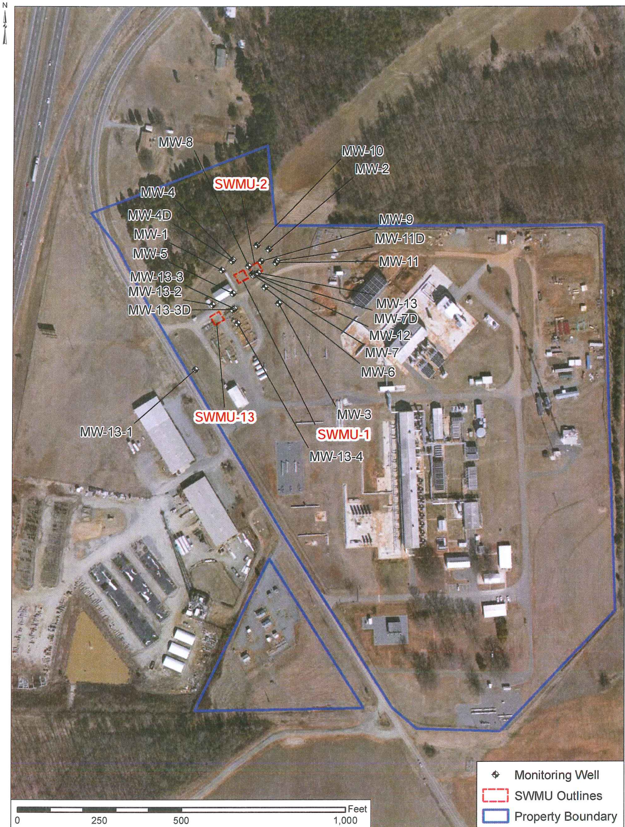
Figure 2 Monitoring Well Location Map
