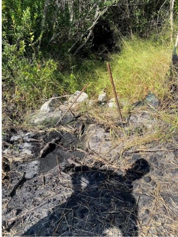
Photo - Overwhelmed TRSC-A with minor sediment loss at Borrow Pit. (9/23/21)
