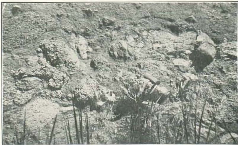
A. Boulders of schist in the Sanford formation. View in cut of the Norfolk Southern Railroad east of Corinth. The boulders are badly decayed, but range in diameter up to 16 inches.
