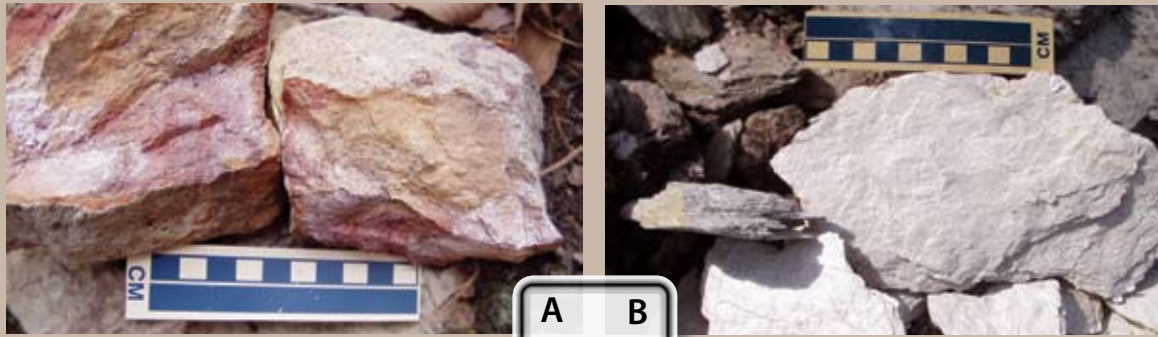
Figure 12 – Photographs of hydrothermally altered rock. A is an example of a sericite and quartz rock with red and yellow mottling.
