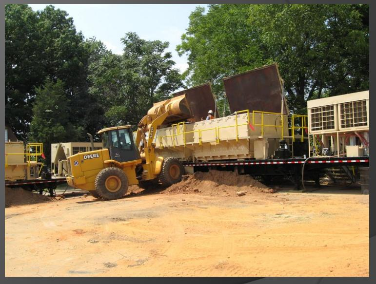
Treated on-site using mobile steam distillation unit
