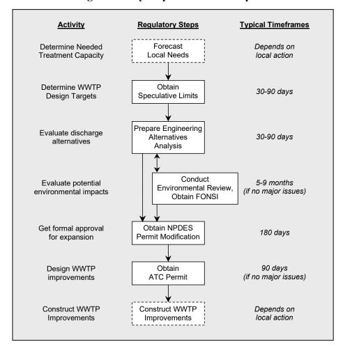
Figure 1. Key Steps for WWTP Expansion
