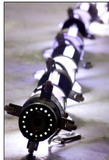
Figure 4-9. UV Light Train for Curing CIPP Liner (Courtesy Reline America, Inc.)
