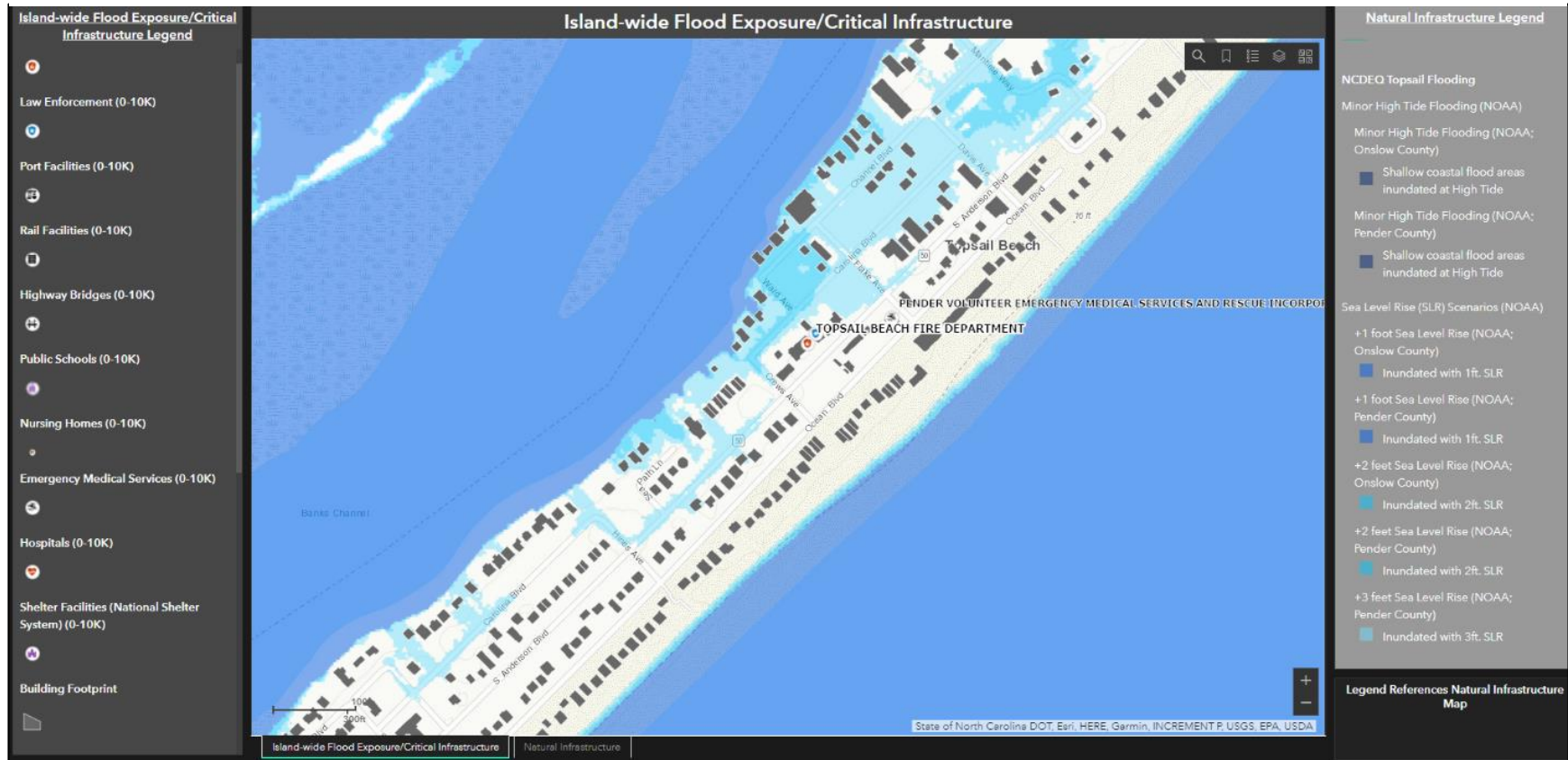
FIGURE A.20 – EXPOSURE TO INCREASING SOUND SIDE NUISANCE TIDAL FLOODING WITH SEA LEVEL RISE (+1, +2 FEET SLR) NEAR WARD AVE. LIVING SHORELINE PILOT SITE IN TOPSAIL BEACH
