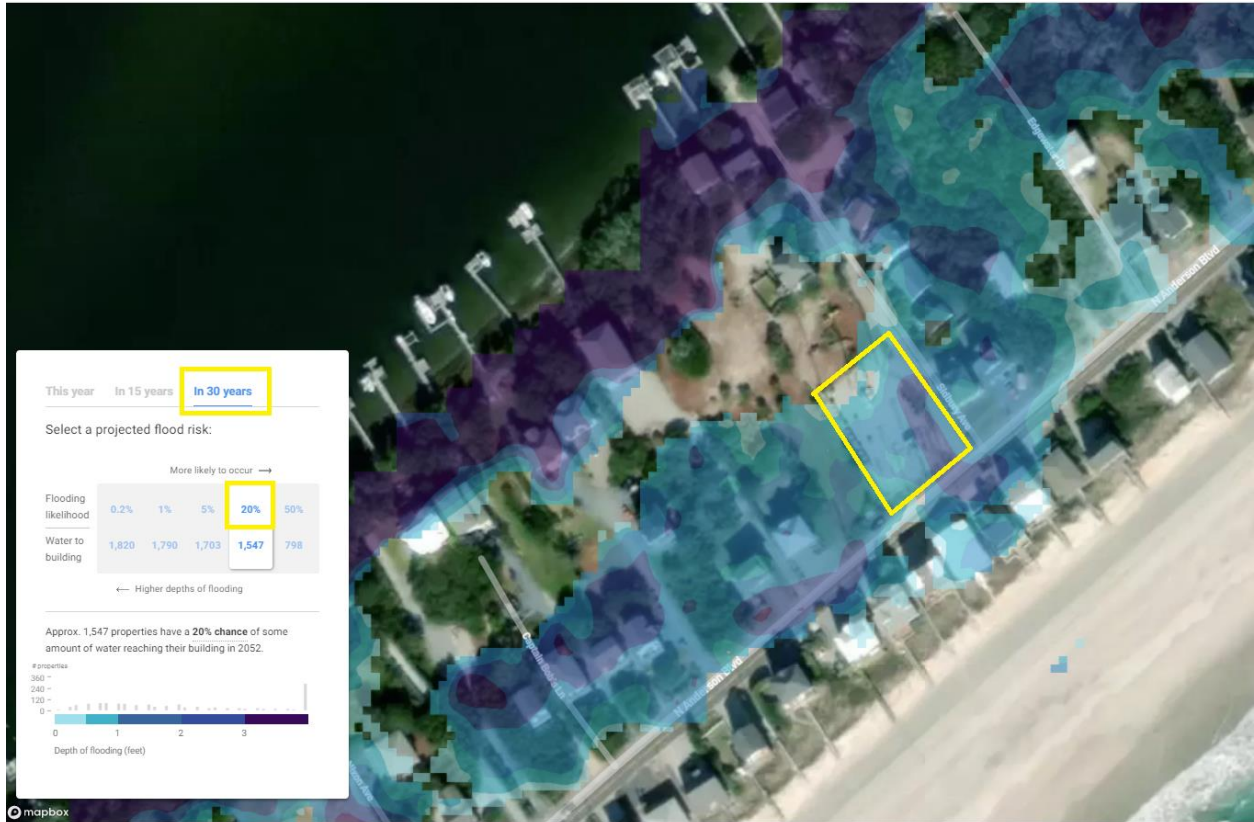
FIGURE B.8 – Modeled 20% event (i.e., 5-year recurrence) flooding in 2050 in Topsail Beach near Sidbury Ave. and electrical substation (source: First Street Foundation FloodFactor https://floodfactor.com/city/topsail-beach-northcarolina/3768040_fsid )
