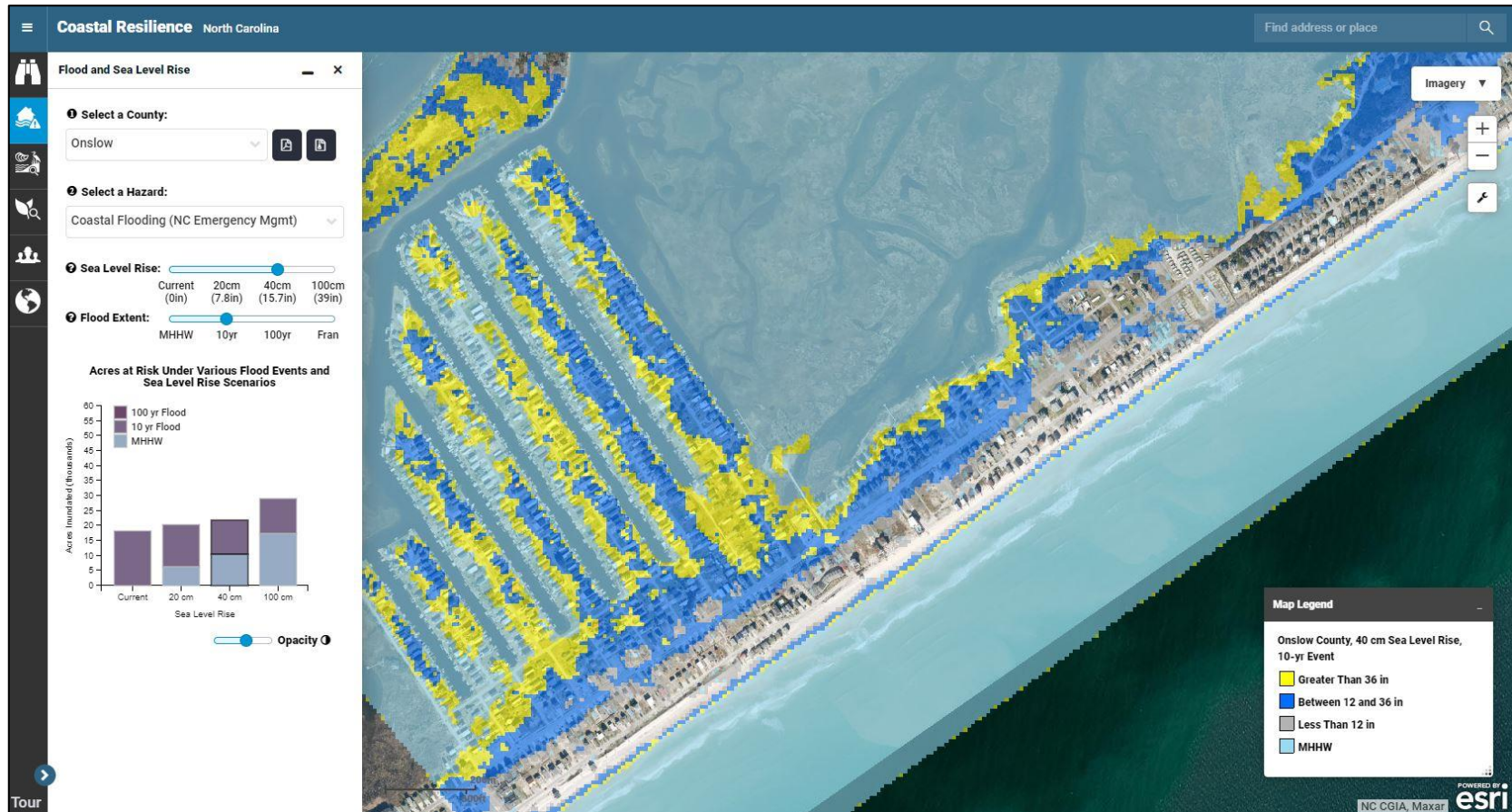
FIGURE A.16 – With additional sea level rise (between +1 to +1.5 feet by 2040-2060, shown in graphic), a 10-year storm event would cause significant sound side flooding along main evacuation routes and isolate entire residential communities, such as those in Surf City near the county line.
