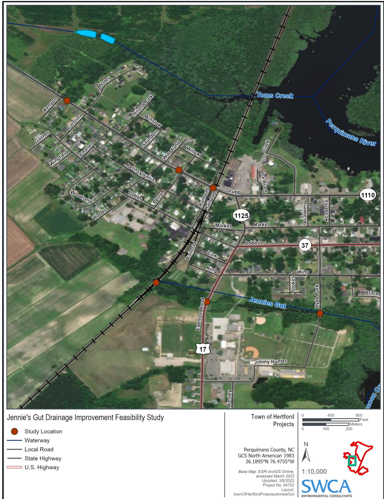
Figure 9. Drainage improvement feasibility study area in Jennies Gut watershed. Red dots show locations where there are known drainage issues such as undersized culverts that cause roadways and other areas to flood during high water.
