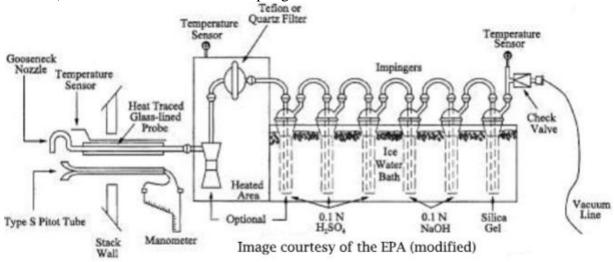
Figure 1 – Schematic of M26A Sampling Train (Courtesy of the EPA)
