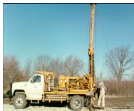
This is one type of auger drilling rig.
