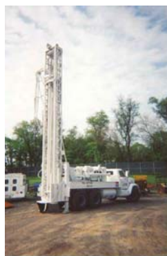
A compressed air drill rig with its drilling tower up.
