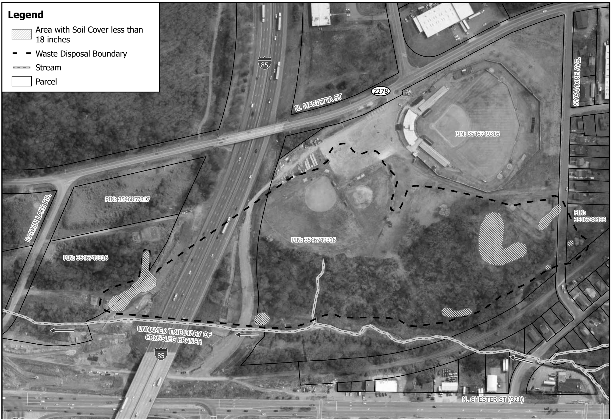
Figure 3: Cover Soil Thickness Sims Legion Park Landfill Gastonia, Gaston County, North Carolina Site Identification Number: NONCD0000766
