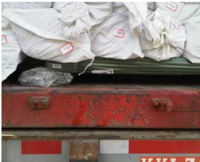
Figure 5-5-2 Example of Inadequate Spacing Under Bamboo Bundles
