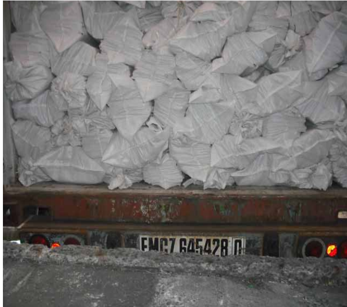
Figure 5-5-1 Example of Inadequate Spacing Under Bamboo Bundles
