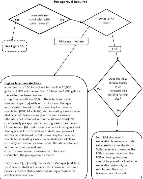
Figure 10 - Soil Excavation for Initial Abatement of a NEW COMINGLED Release at a Site with a Prior Release AND Risk Ranking AND USTs are Being Permanently Closed (or do not impede soil excavation) - Pre-approval Required
