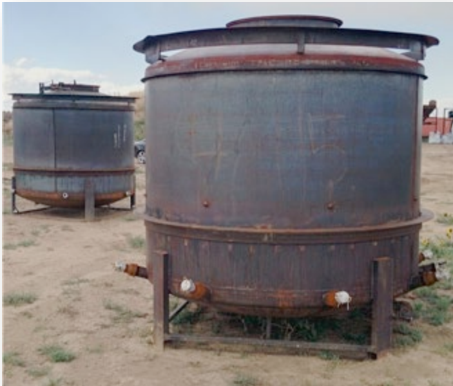
Biochar Kilns Dimensions: ~7.5 feet in Diameter ~8 feet in height
