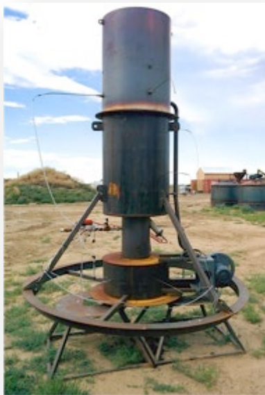
Afterburner Stack Dimension: ~8 feet in height
