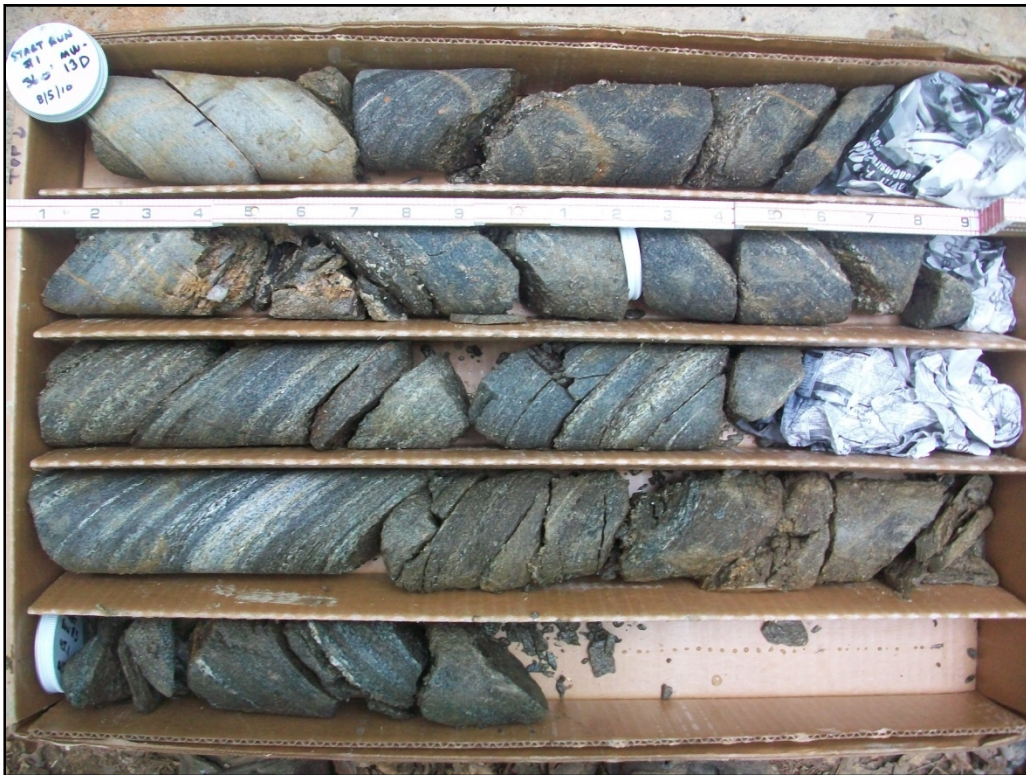
Photo 20: MW-13D, Entire Core including Run #1 (36.0 – 40.2 ft.), Run #2 (40.2 – 45.1 ft.) and Run #3 (45.1 – 46.4 ft.)
