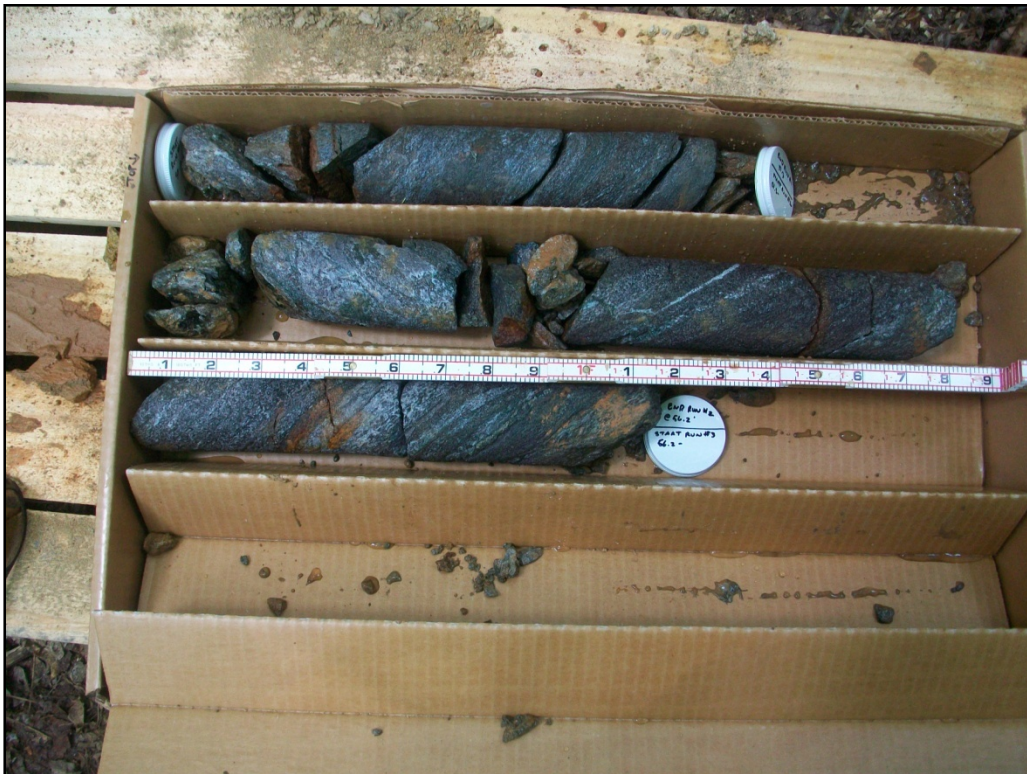
Photo 6: MW-14D, Core Run #2 (51.3 – 56.2 ft.)
