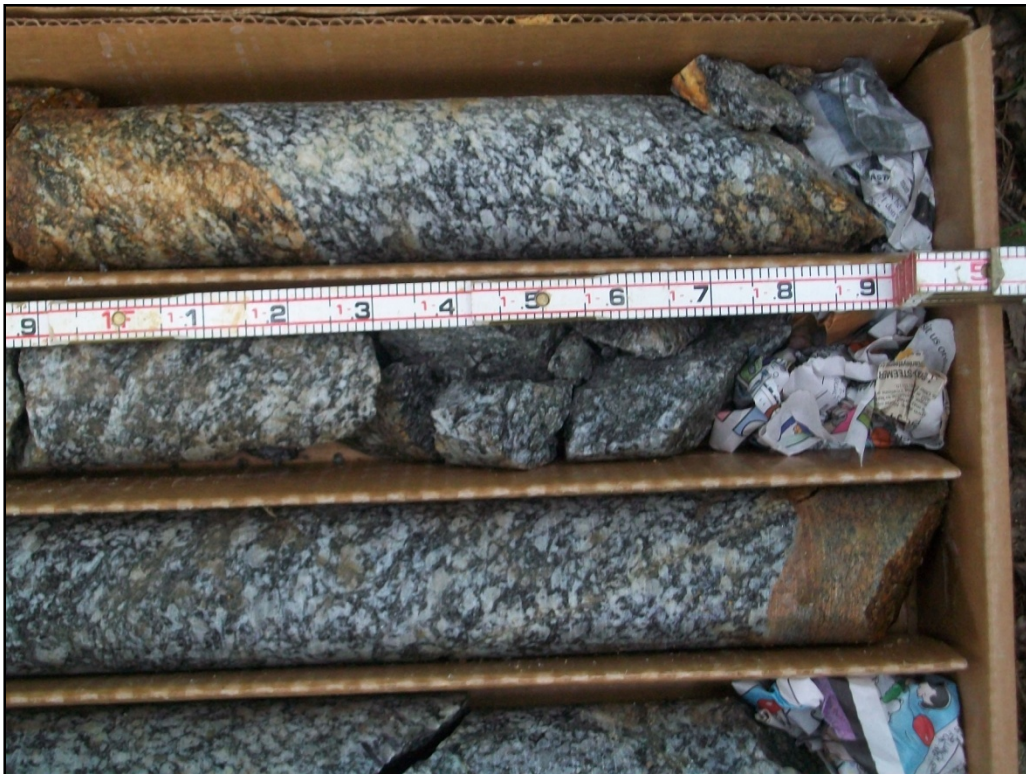
Photo 12: MW-12D, Bottom of Core Runs #1 (94.0 – 96.2 ft.) and #2 (96.2 – 101.5 ft.)
