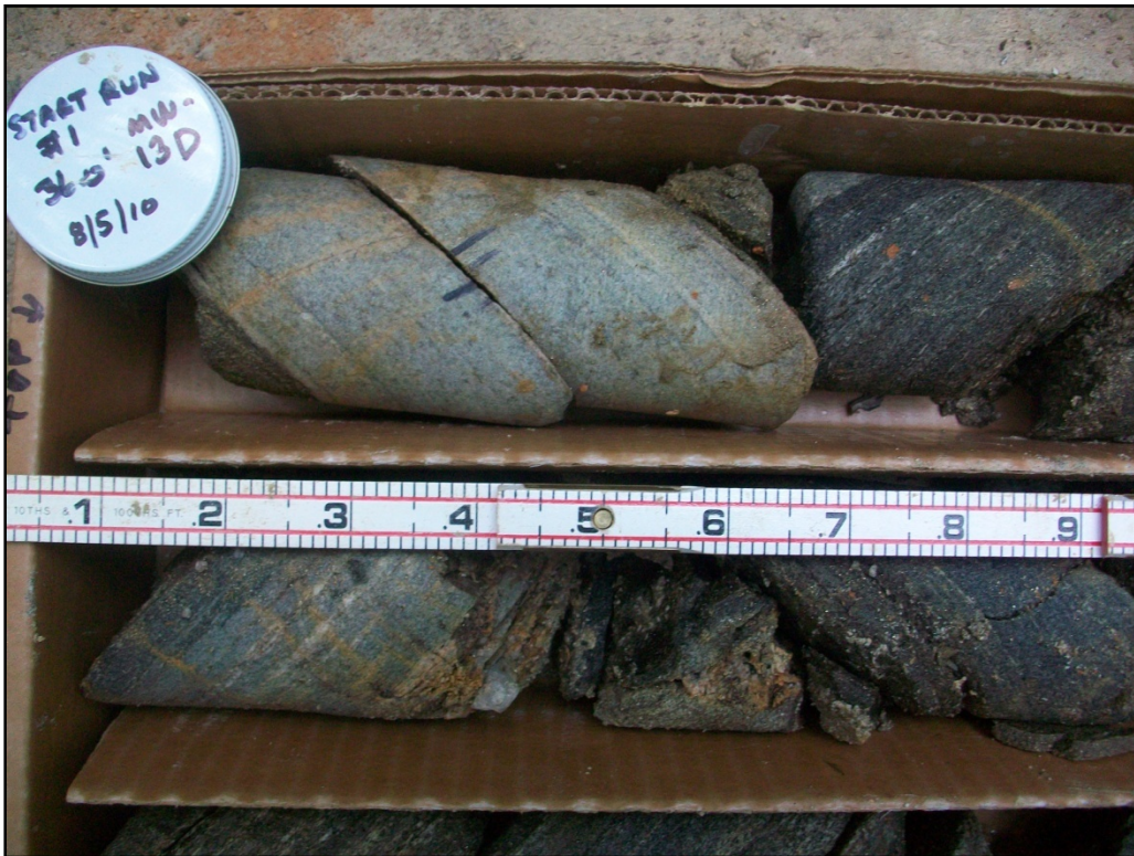
Photo 16: MW-13D, Core Run #1 (36.0 – 40.2 ft.)
