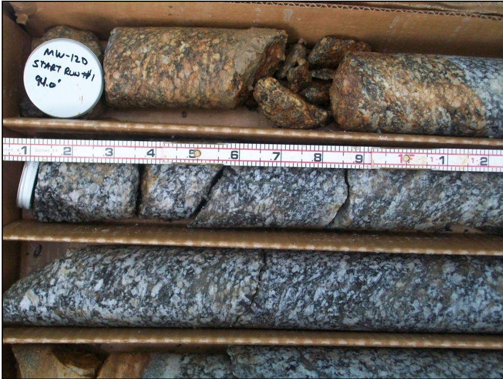
Photo 11: MW-12D, Top of Core Runs #1 (94.0 – 96.2 ft.) and #2 (96.2 – 101.5 ft.)
