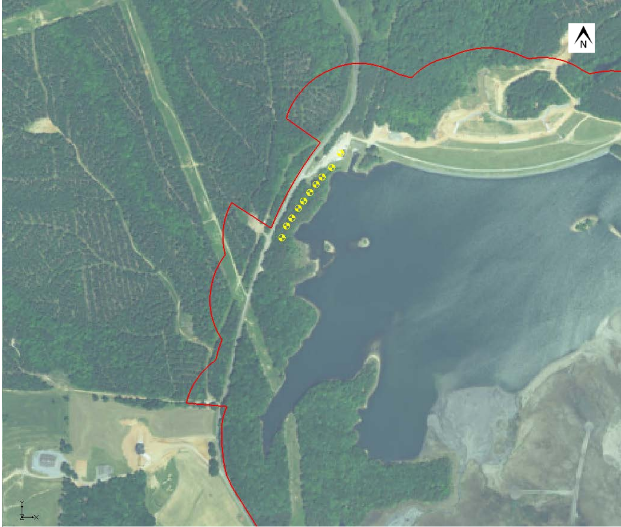
Figure 6-1. Location of current accelerated remediation wells. The red line is the compliance boundary and the yellow circles are the 10 interim action groundwater extraction wells. The red outline is the compliance boundary.
