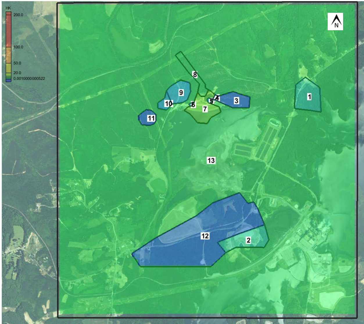
Figure 5-5. Zones used to define horizontal hydraulic conductivity and horizontal to vertical anisotropy in the transition zone, model layer 15.
