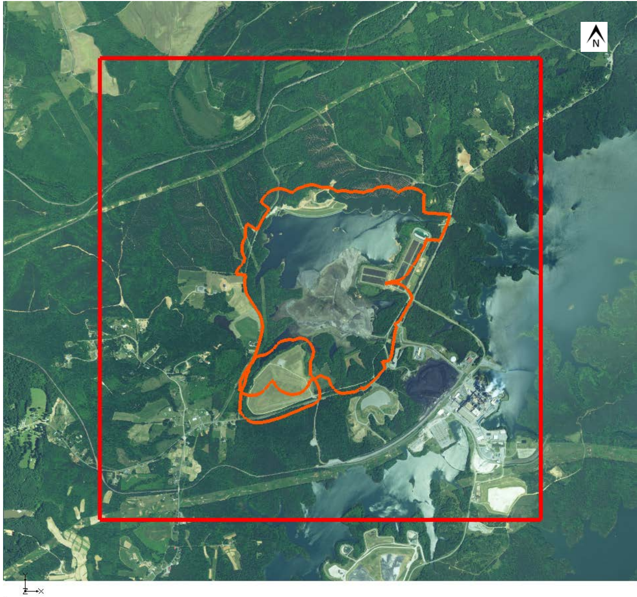
Figure 4-1. Numerical model domain. Domain is represented as the red square. The larger orange outline is the ash basin compliance boundary and the smaller orange outline is Pine Hall Road Landfill.
