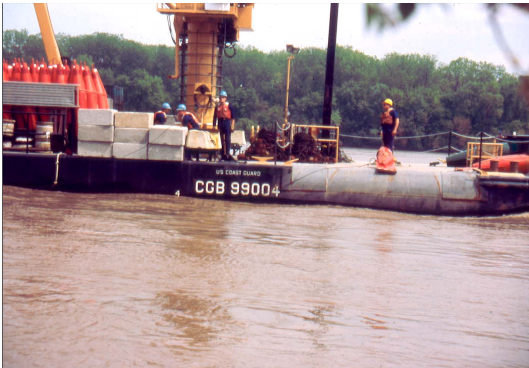
Buoy to Bank Anchor System USCG Buoy Tender in Position to Drop 1600 lb. Sinker with Buoy Missouri River - St. Louis, Missouri Area
