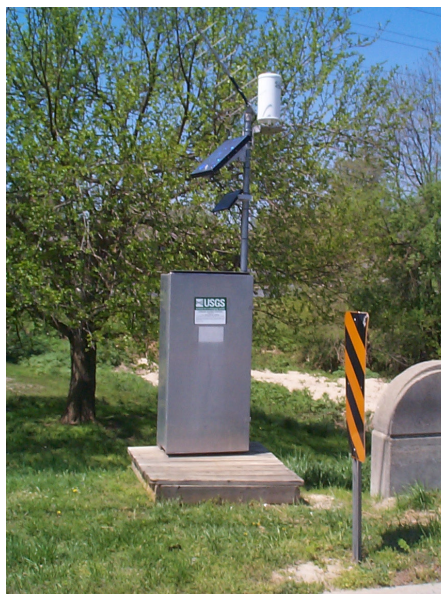
USGS stream flow and precipitation gaging station on North Buffalo Creek at Church Street. This and other gaging stations in the area are operated with support from Greensboro's Department of Water Resources.
