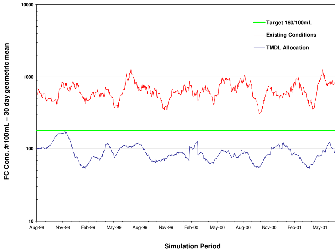
Figure 4.5.2 Predicted geometric mean fecal coliform concentration at Summit Avenue before and after load reductions were applied to the calibrated model.
