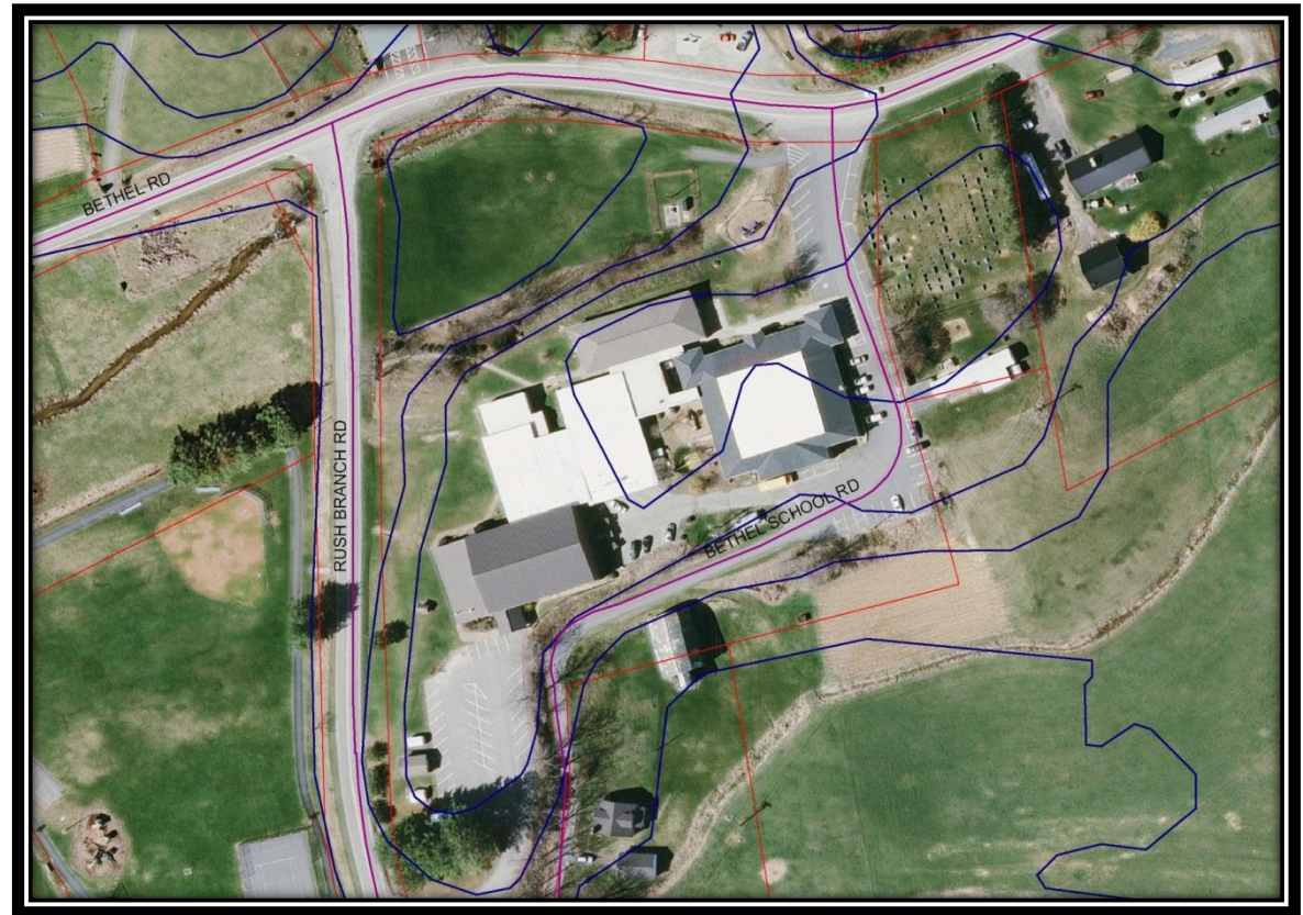
Figure 8: Aerial photo of Bethel Elementary School showing extent of rooftops and parking with contours shown in blue.
