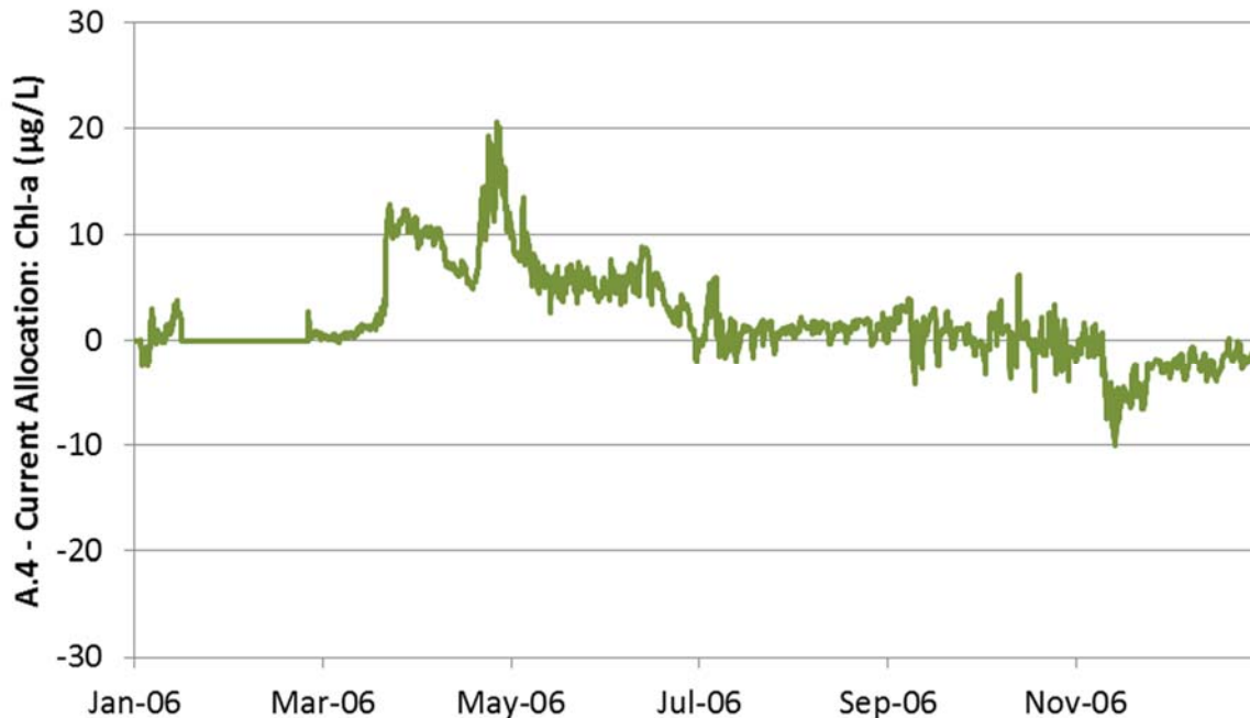
Figure 7: Difference between A.4 allocation Chl-a concentrations and those simulated for the current allocation at the NEU013B compliance point
