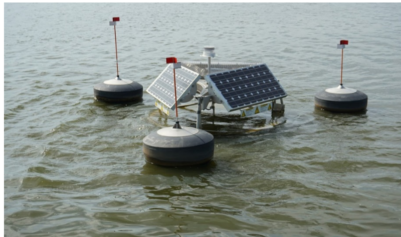
Solar-powered surface-layer circulator on Jordan Lake
