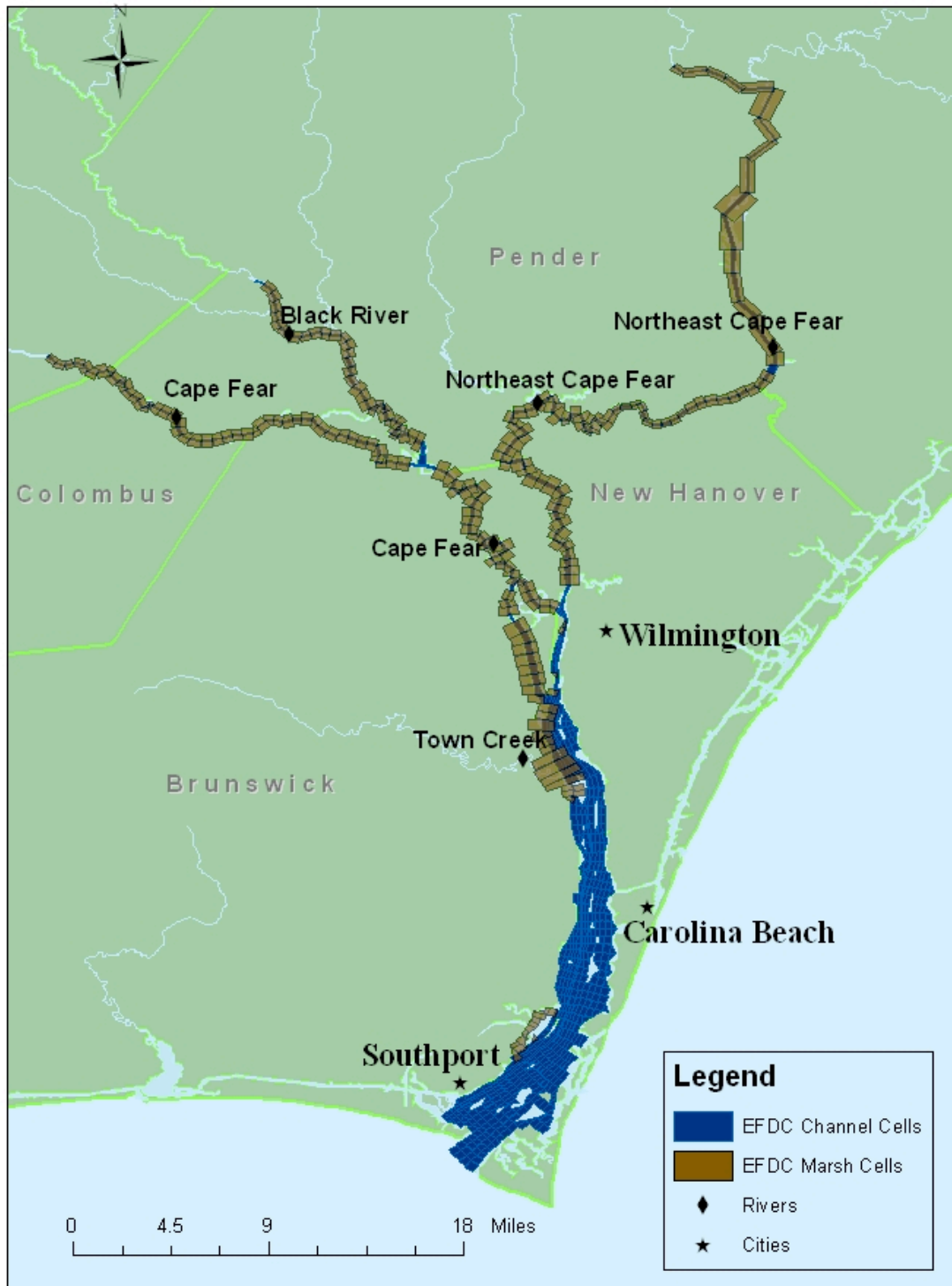
Figure 6. Model Grid Showing Location and Size of Marsh Cells
