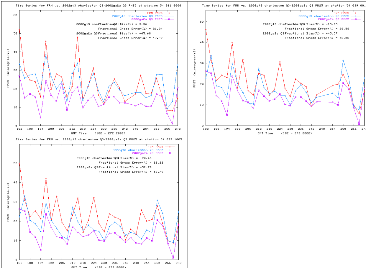
Figure D-18c. (continued) Time Series of predicted and observed 24-hour PM 2.5 concentrations for FRM sites in the Charleston subdomain, Quarter 3 and the CAMx 2002gt3 and CMAQ 2020aga2 base case simulations.
