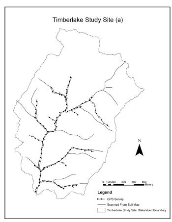
Figure 2. Comparison of streams shown on USGS 1:24,000 scale topographic map to GPS ground truth in a watershed in Person County, NC.
