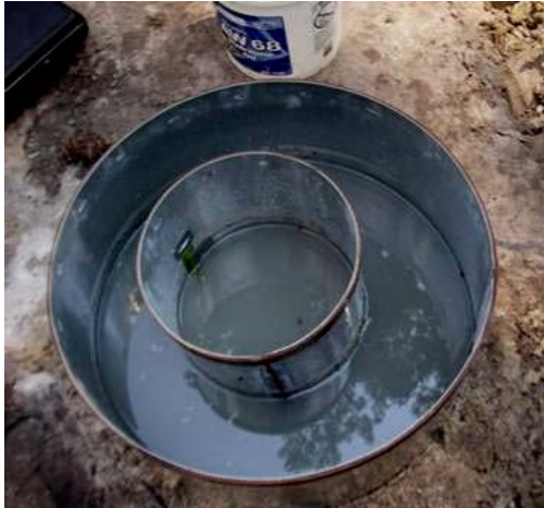
Figure 18-6a. Double ring infiltration tests apparatus Source: NCSU-BAE
