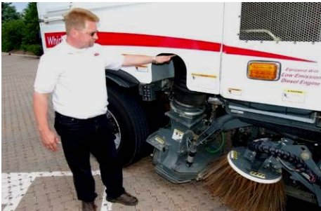
Figure 18-26. A true vacuum truck can help restore infiltration to severely clogged permeable pavement. Source: NCSU-BAE
