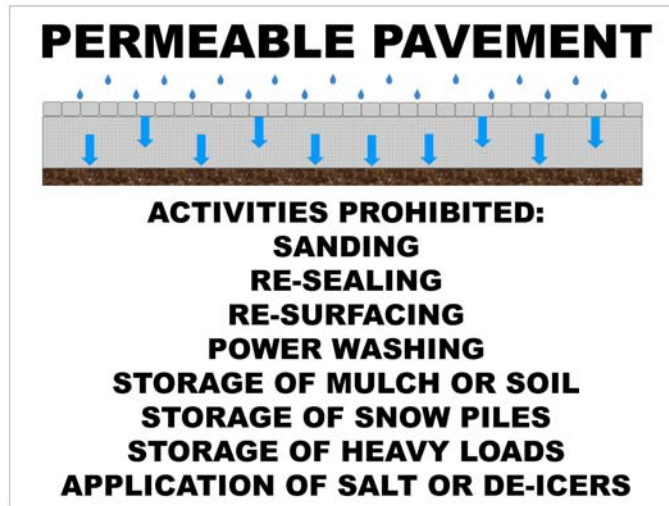
Figure 18-14. Example sign layout for permeable pavement sites
