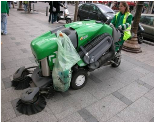
Figure 18-24. Sweeper equipment for cleaning sidewalks Source: NCSU-BAE
