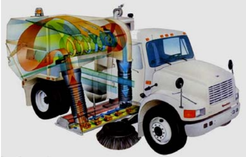
Figure 18-25. Regenerative air vacuum truck Source: TYMCO, Inc.
