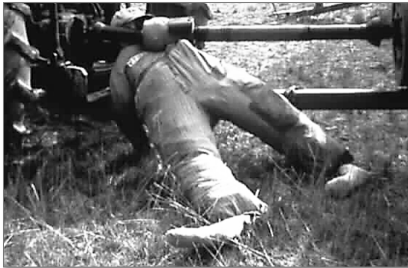
Figure 11-5. Mock demonstration of a wrapping injury caused by a PTO device.
