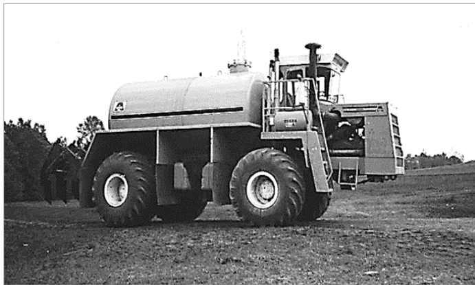
Figure 9-13. Self-propelled, high flotation vehicle with tank for liquid residuals.
