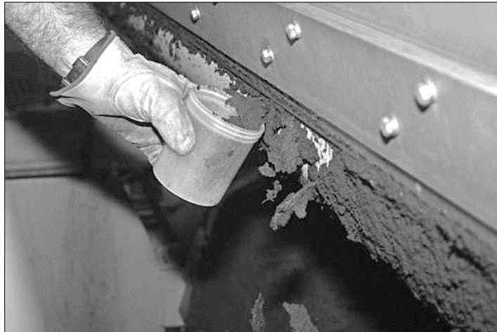
Figure 14-4. Sampling dewatered residuals as they are dropping into belt press hopper.
