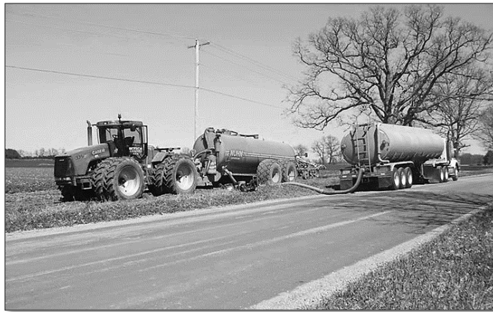
Figure 9-12. Residuals being transferred from “nurse” truck to application vehicle.
