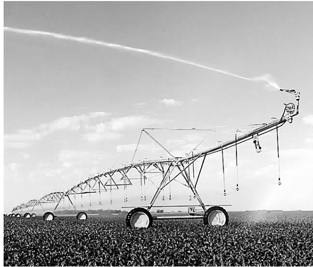
Figure 4-18. Center pivot system.
