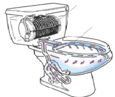
Pressure Assisted Toilet
